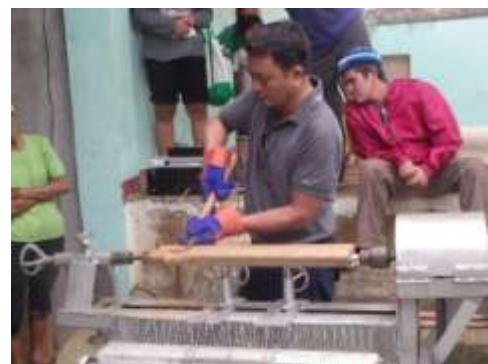
Figure 12. Testing the wood working machine in making broom handle
